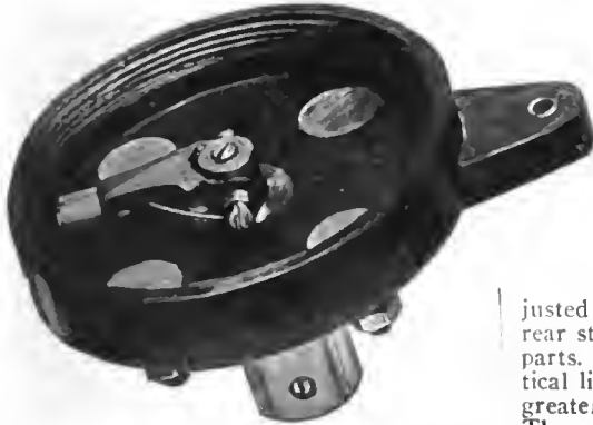
DODGE POSITIVE TIMER, SHOWING ROTATING ARM AND CONTACT PLATES.
